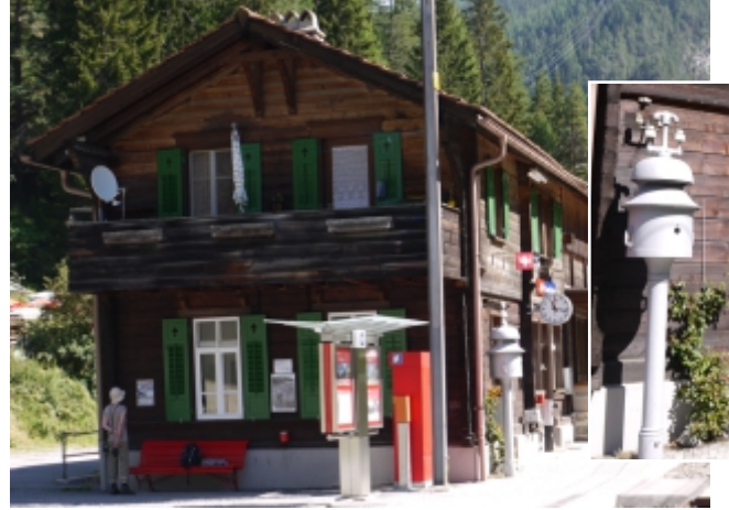
Wiesen (above) and Ospizio Bernina (down) have signal bells with insulators.
