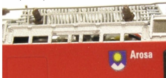
Chassis with glued Zimo MX616 decoder. When the housing is attached, the decoder fits under the cover on top of the roof and is practically invisible.
