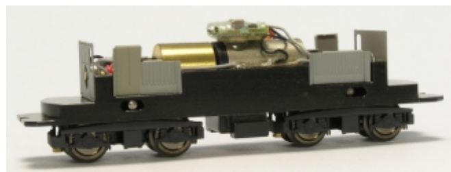
Chassis with glued Zimo MX616 decoder. When the housing is attached, the decoder fits under the cover on top of the roof and is practically invisible.
